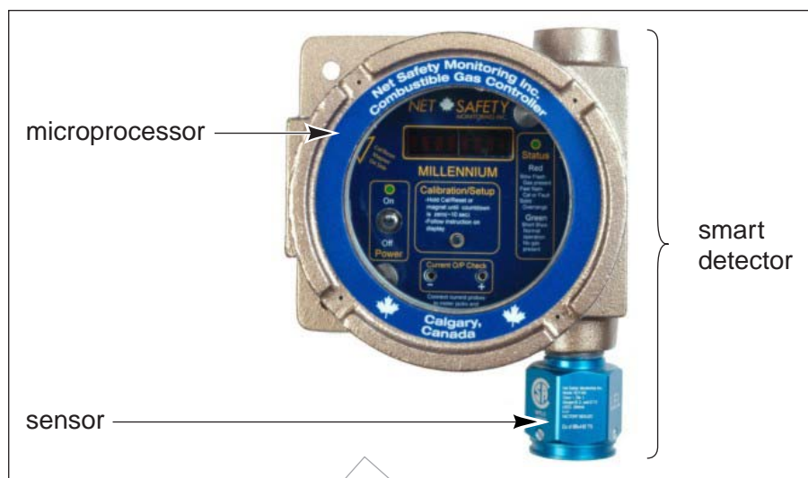
Figure 7— Fixed Catalytic Combustion Detector
